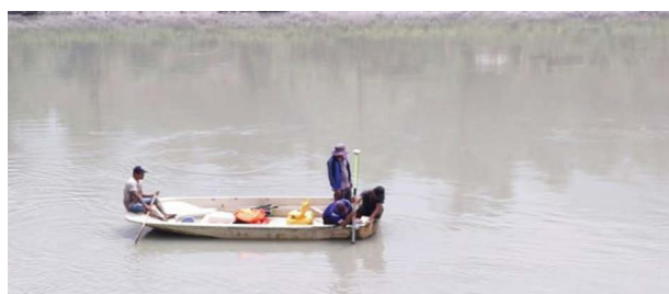
Figure 3: Bathymetric Surveying in Lower Marshyangdi Reservoir
