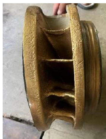
Damaged Bronze Runner during Overhauling
