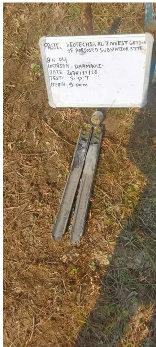
Soil Sample in Split Spoon Sampler of New Borehole 4 of Damauli SS; Depth 9 m
