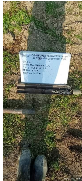
Soil Sample in Split Spoon Sampler of New Borehole 3 of Damauli SS; Depth 4.5 m
