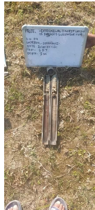
Soil Sample in Split Spoon Sampler of New Borehole 4 of Damauli SS; Depth 3 m
