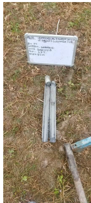
Soil Sample in Split Spoon Sampler of New Borehole 4 of Damauli SS; Depth 7.5 m
