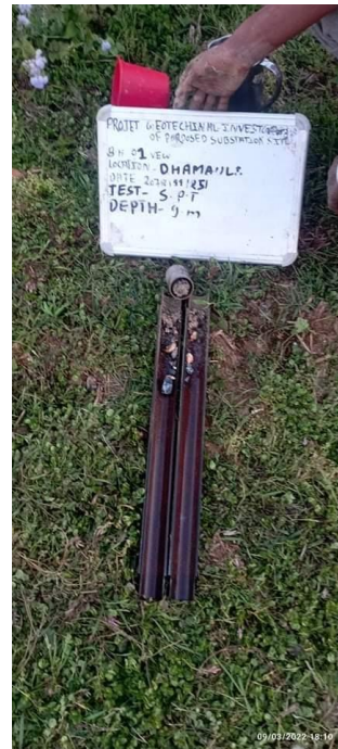
Soil Sample in Split Spoon Sampler of New Borehole 1 of Damauli SS; Depth 9 m
