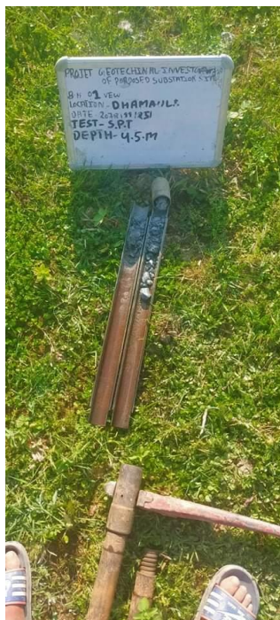
Soil Sample in Split Spoon Sampler of New Borehole 1 of Damauli SS; Depth 4.5 m
