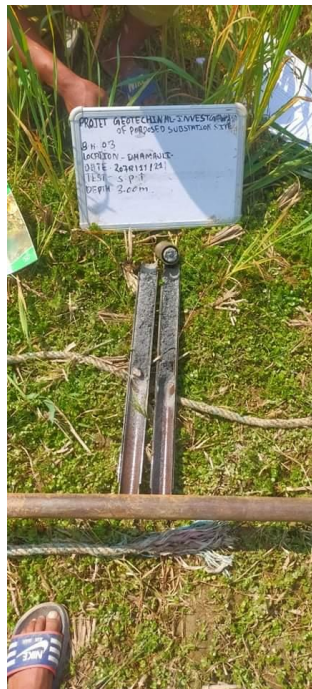
Soil Sample in Split Spoon Sampler of New Borehole 3 of Damauli SS; Depth 3 m
