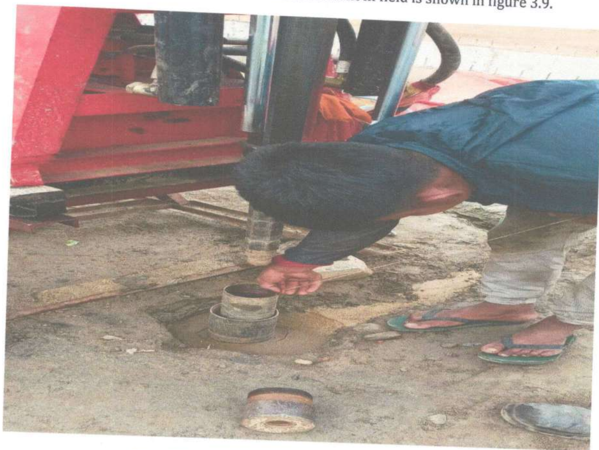
Figure 3-9 Ground water table measurement in field at BH-01
