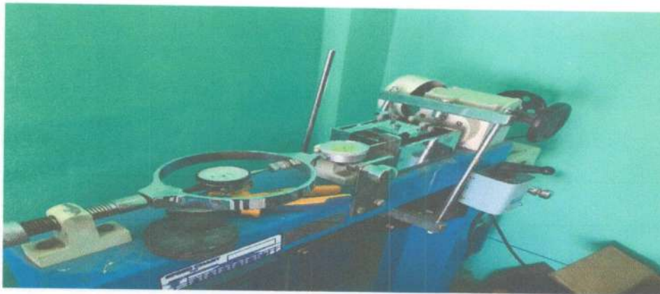
Figure 3-10 Direct Shear Test arrangement
