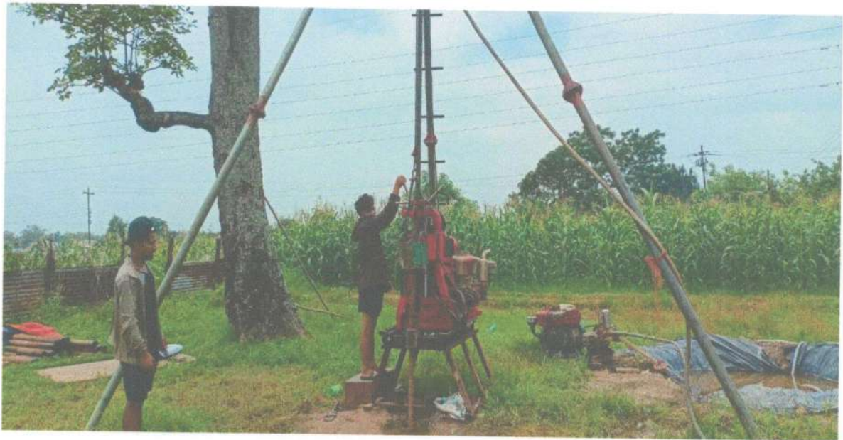
Figure 3-1 SPT test arrangement and rotatory bore hole drilling arrangement at BH-01
