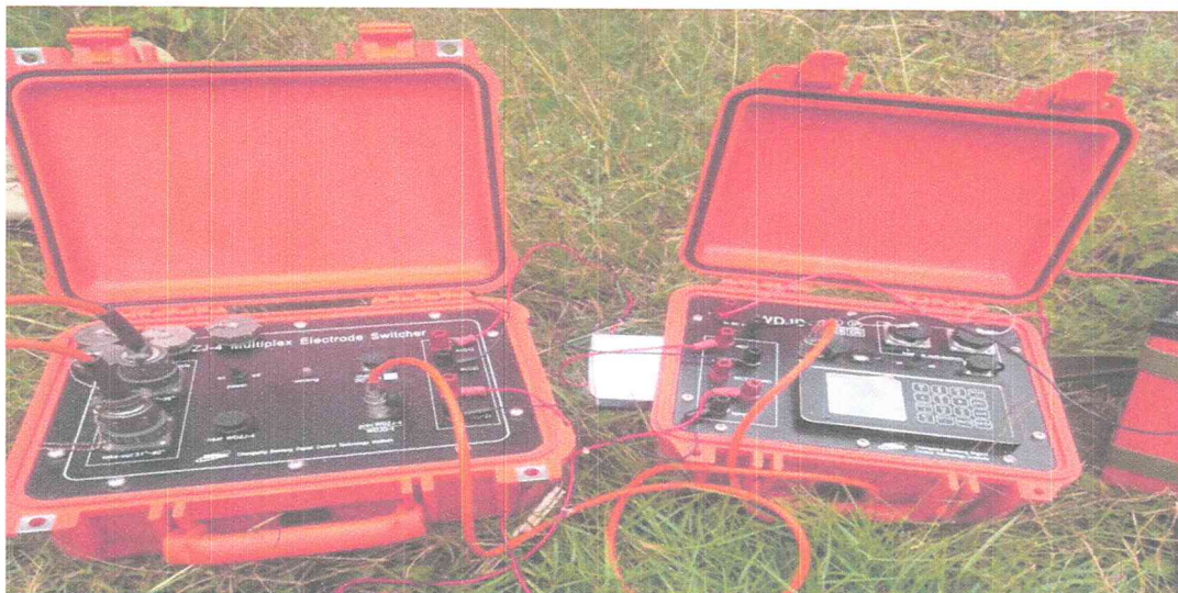
Figure 2: Multi-function digital DC Electrical Resistivity meter.
